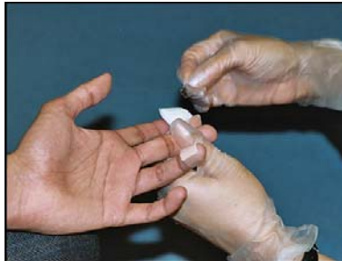
Figure 6.4 Filling and wiping the outside of the microcuvette
